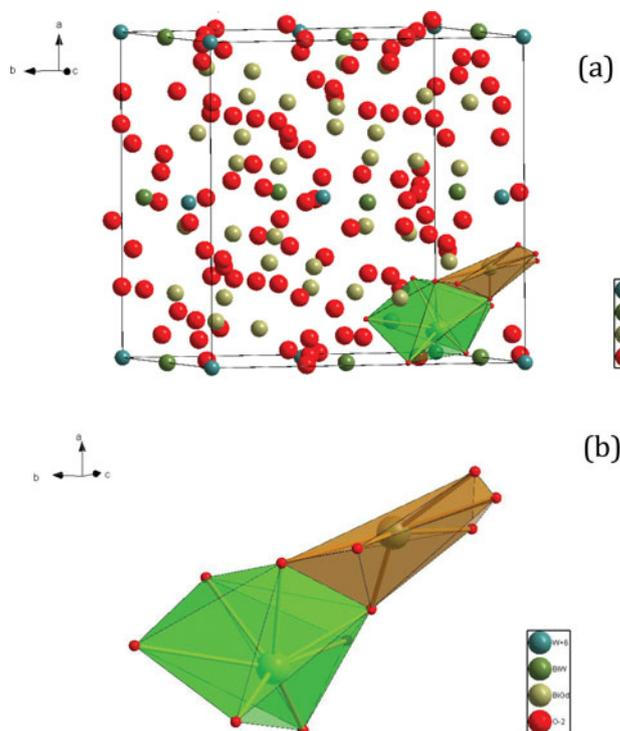
**Figure 3.** (a) Crystal Structure of  $(\text{Bi}_{1-x}\text{Gd}_x)_{14}\text{W}_2\text{O}_{27}$  (space group  $I4_1/a$ ) with Bi/Gd in the 6-fold and 7-fold coordinations and (b) representation of the polyhedra without the  $6s^2$  lone pair electrons due to Gd substitution.
