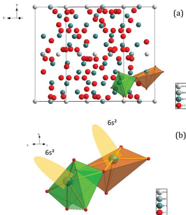
**Figure 2.** (a) Crystal Structure of  $\text{Bi}_{14}\text{W}_2\text{O}_{27}$  (space group  $I4_1/a$ ) with Bi in the 5-fold and 6-fold coordination and (b) representation of the polyhedra with the  $6s^2$  lone pair electrons.
