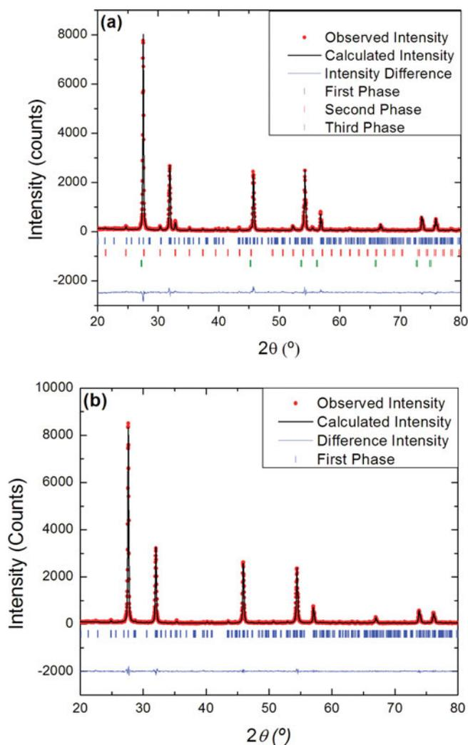
**Figure 1.** Rietveld refinement of (a)  $\text{Bi}_{14}\text{W}_2\text{O}_{27}$  and (b)  $(\text{Bi}_{0.95}\text{Gd}_{0.05})_{14}\text{W}_2\text{O}_{27}$ .
